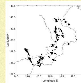
Epicentral map of the seismicity obtained by the earthquake simulator for the first 1000 years.
